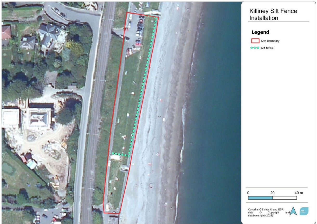
Figure 7-1: The location of the proposed silt fence located along the fence in the east of the site
