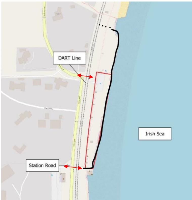
Figure 3-2: Extent of the flood defence designed for people on the crest during overtopping events: defence extent to protect the whole promenade (black line), principal access to the beach (red double arrows)
