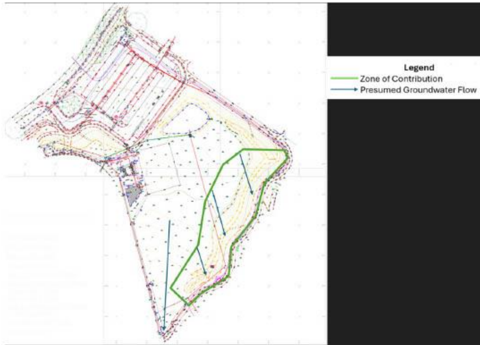
Figure 3.1 Preliminary ZOC based on site topography (no site investigations undertaken to confirm).
