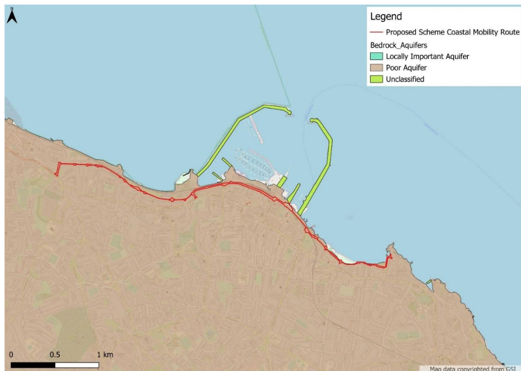
Figure 6. 2: Bedrock Aquifer (Map Source: Geological Survey Ireland)
