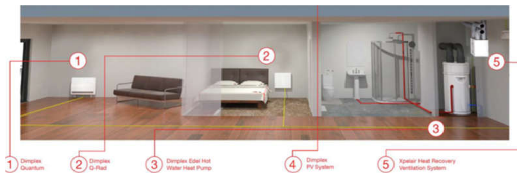
Typical smart electric system.
