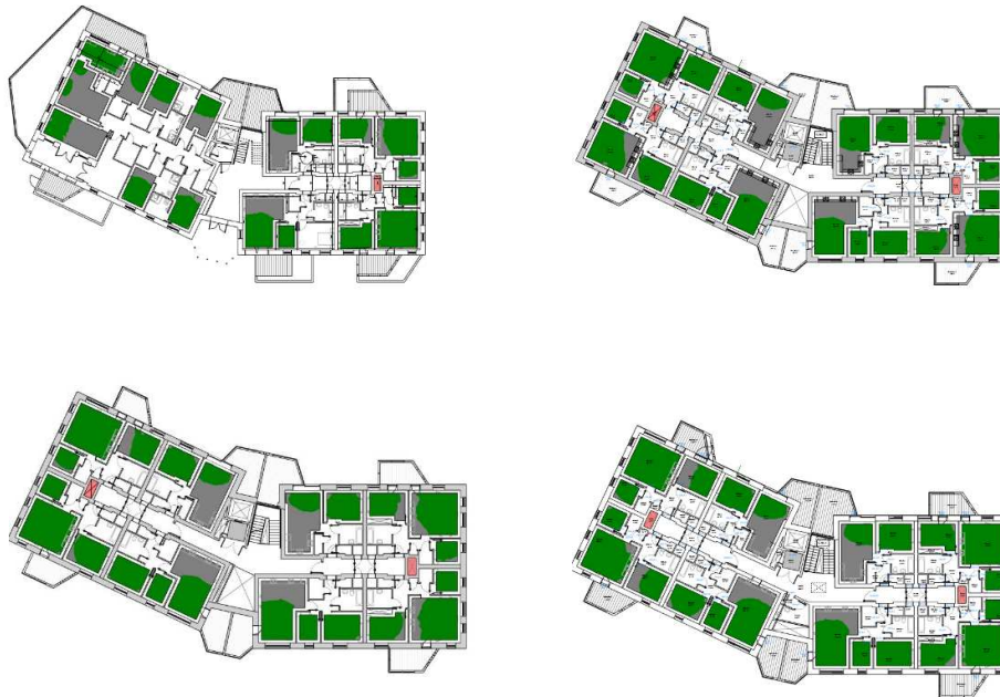
SDA results Block C. top: Grund and First floors, , bottom, 2 nd and third floors
