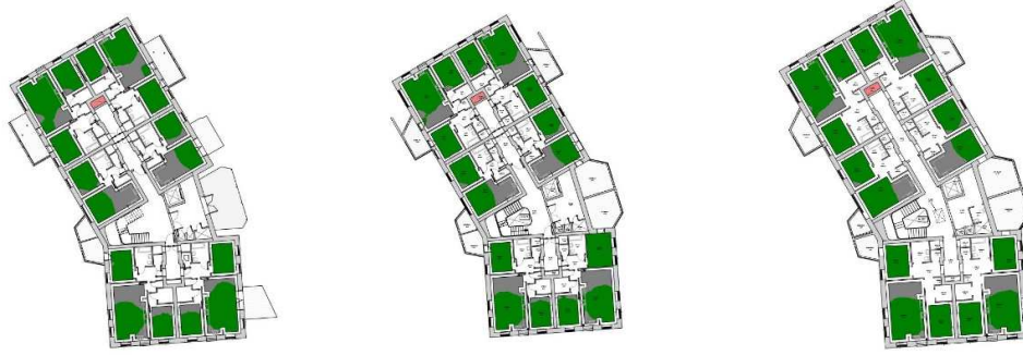
SDA-graphic results to Block A, ground, 1 st and 3 rd floors
