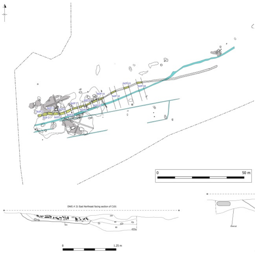
Plan showing the location of slots excavated across the water management area (1-4 and the mater management ditches further east (5-14; top)
