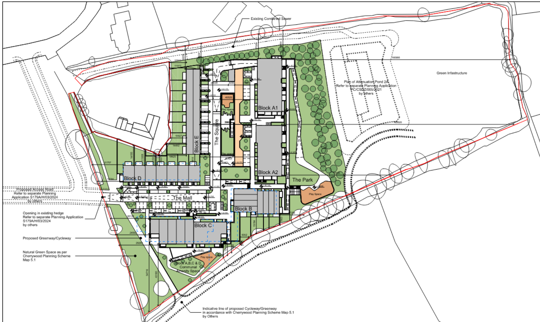
Figure 3-2: Architect's Site Layout ©ABK Architects
