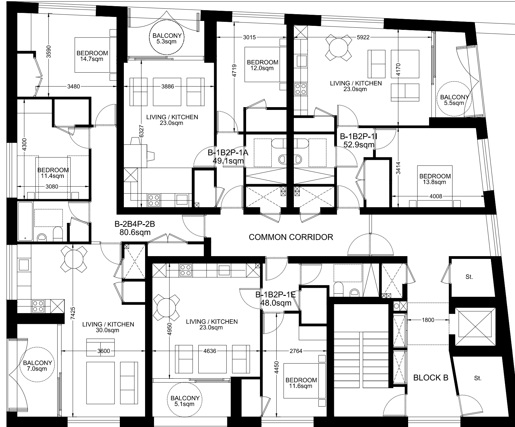
BLOCK B FIFTH FLOOR PLAN
