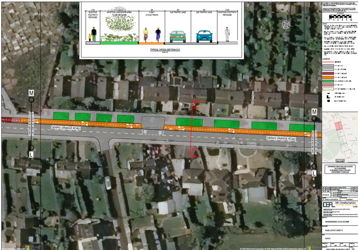
Figure 6 Outline design and layout of proposed scheme- Section 5 (source: DBFL Consulting Engineers)
