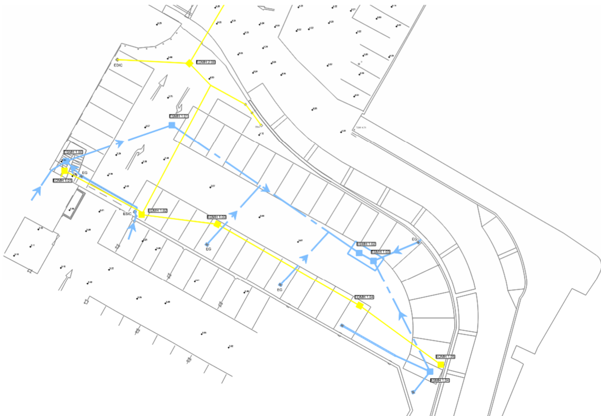
Figure 4-1 - Existing SW Drainage Layout
