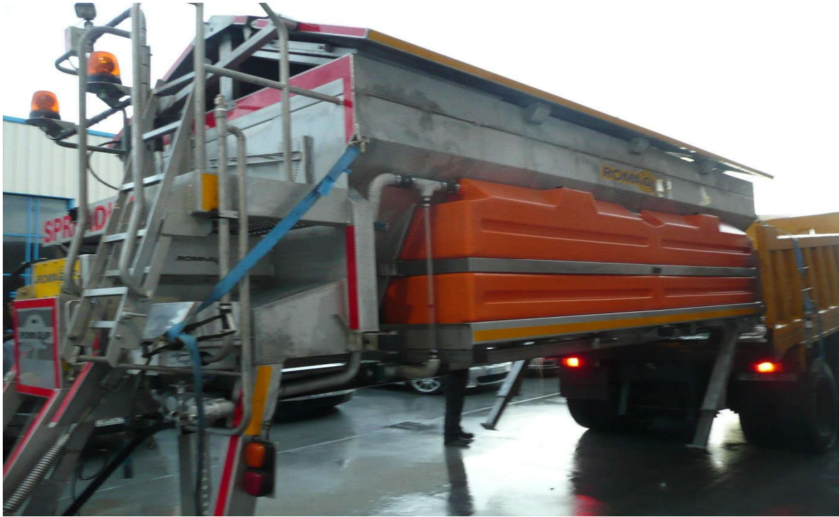
Typical 9m 3 Brine Tank (orange) on a Demountable Gritter
