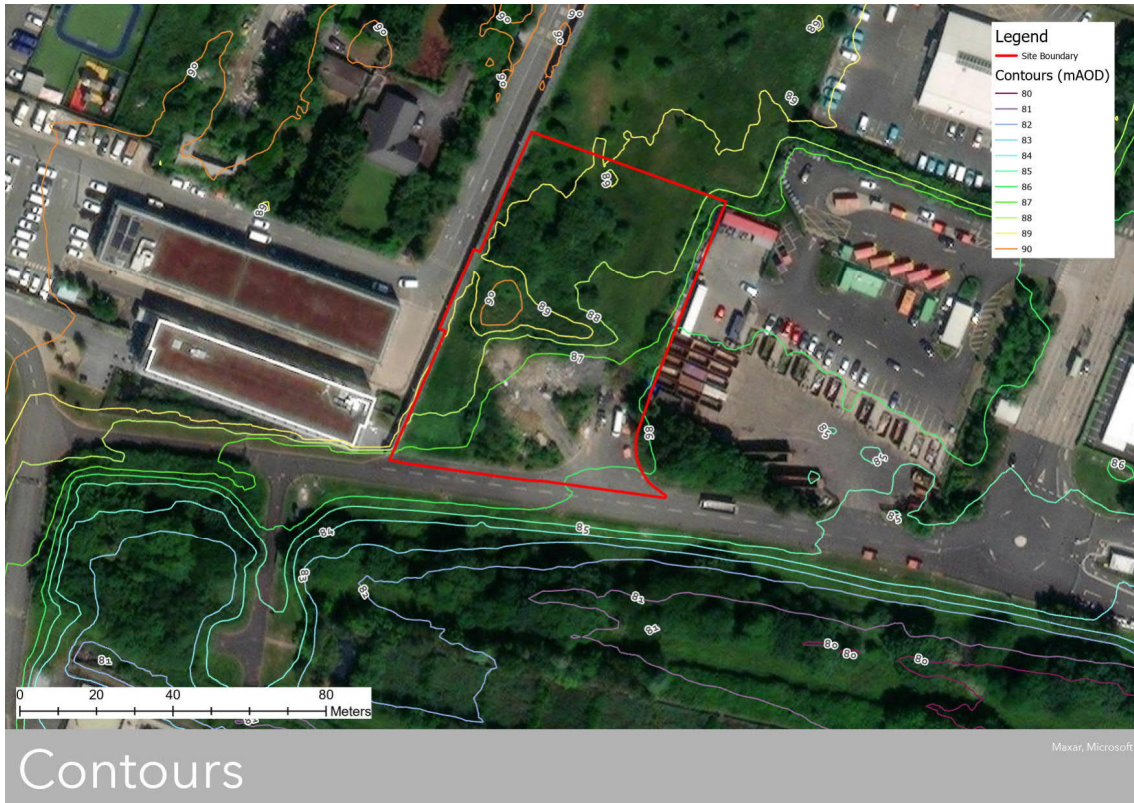
Figure 3-4: Site contours from GSI Open Topographic Data - LiDAR Office of Public Works (OPW) NASC Index: OPW_3285 data, captured 2011
