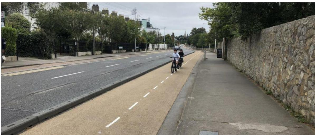
Figure 7-2 Example two-way kerb protected cycle track
