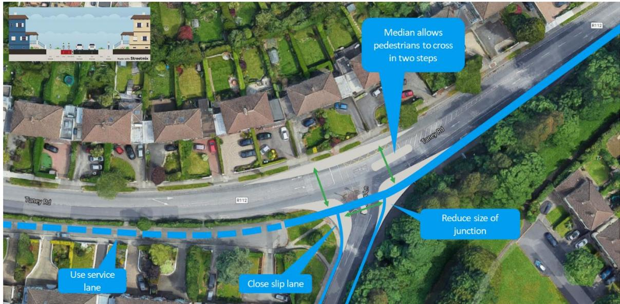
Figure 7-6 Birches Lane: Option 3 (two-way, south side)
