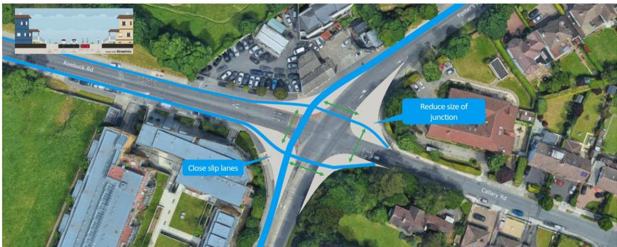
Figure 7-11 Roebuck/Callary Junction: Option 2 (two-way north side)
