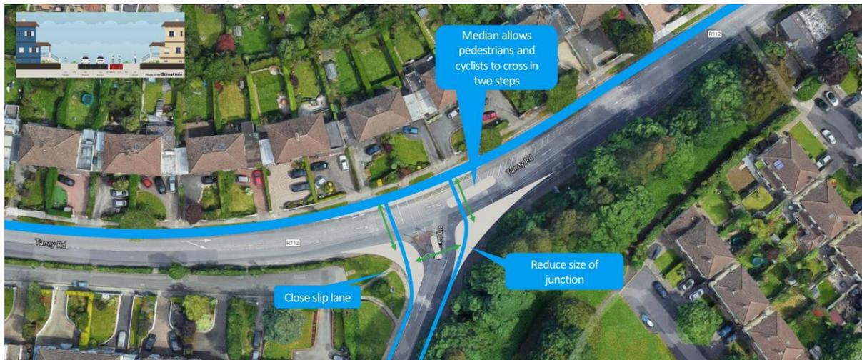
Figure 7-5 Birches Lane: Option 2 (two-way, North side)
