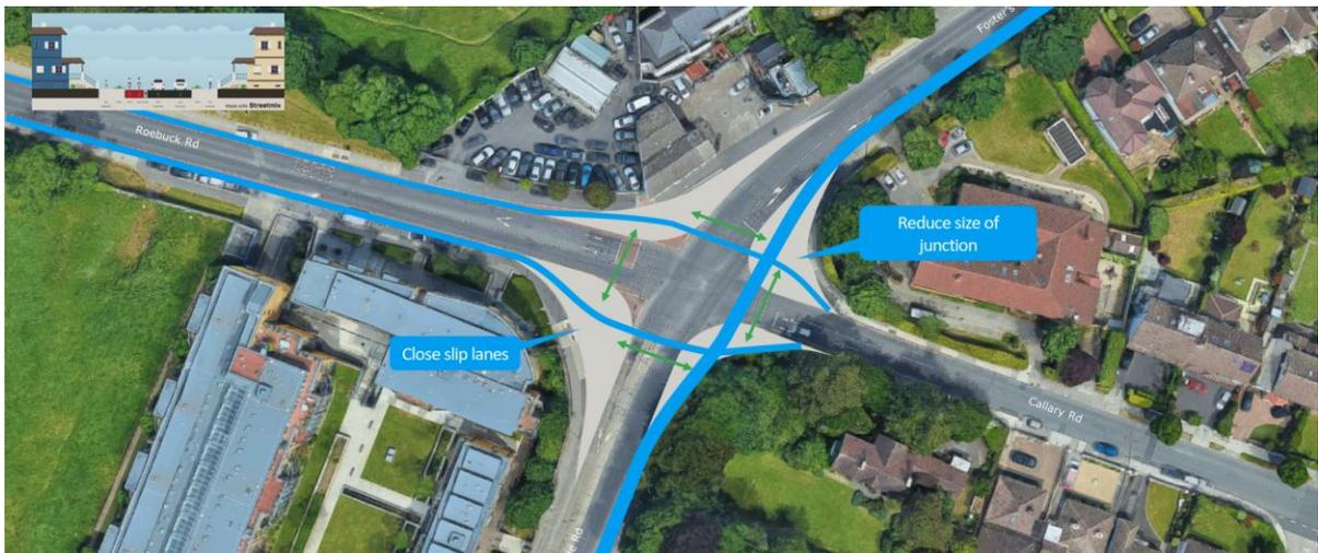
Figure 7-12 Roebuck/Callary Junction: Option 3 (two-way south side)
