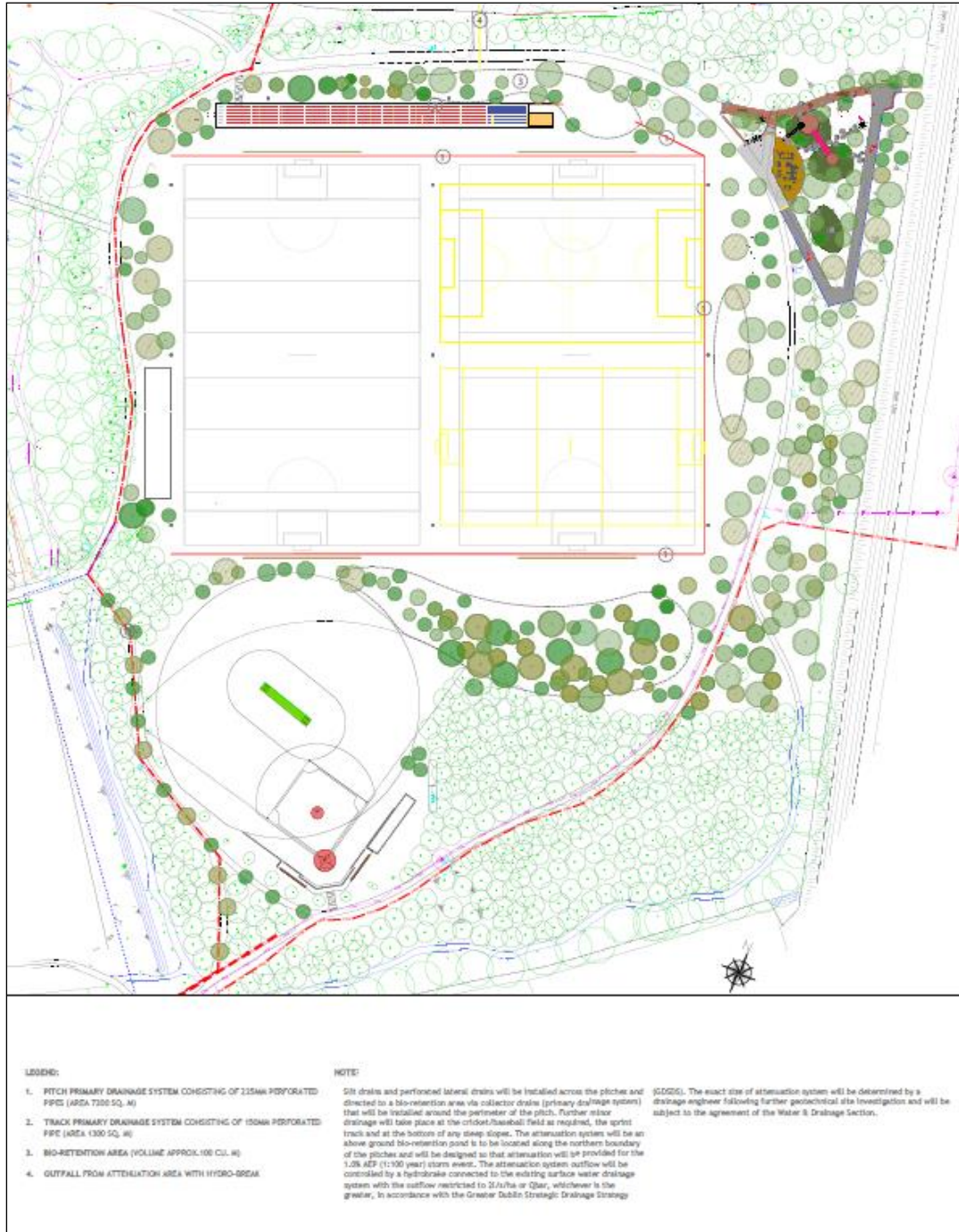
Figure 3 Site Drainage – Drawing no DRP 2422-12
