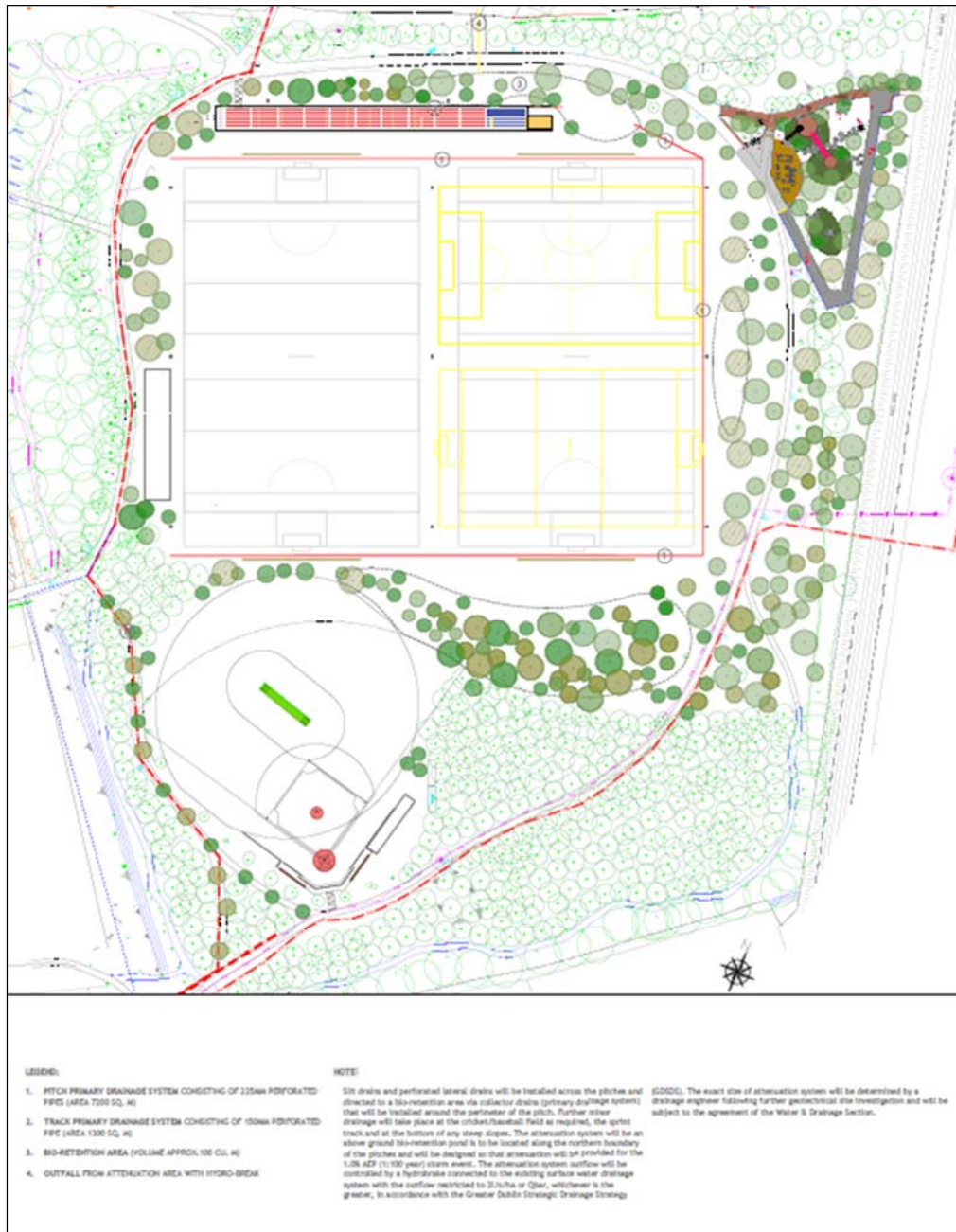
Figure 3 Site Drainage – Drawing no DRP 2422-12
