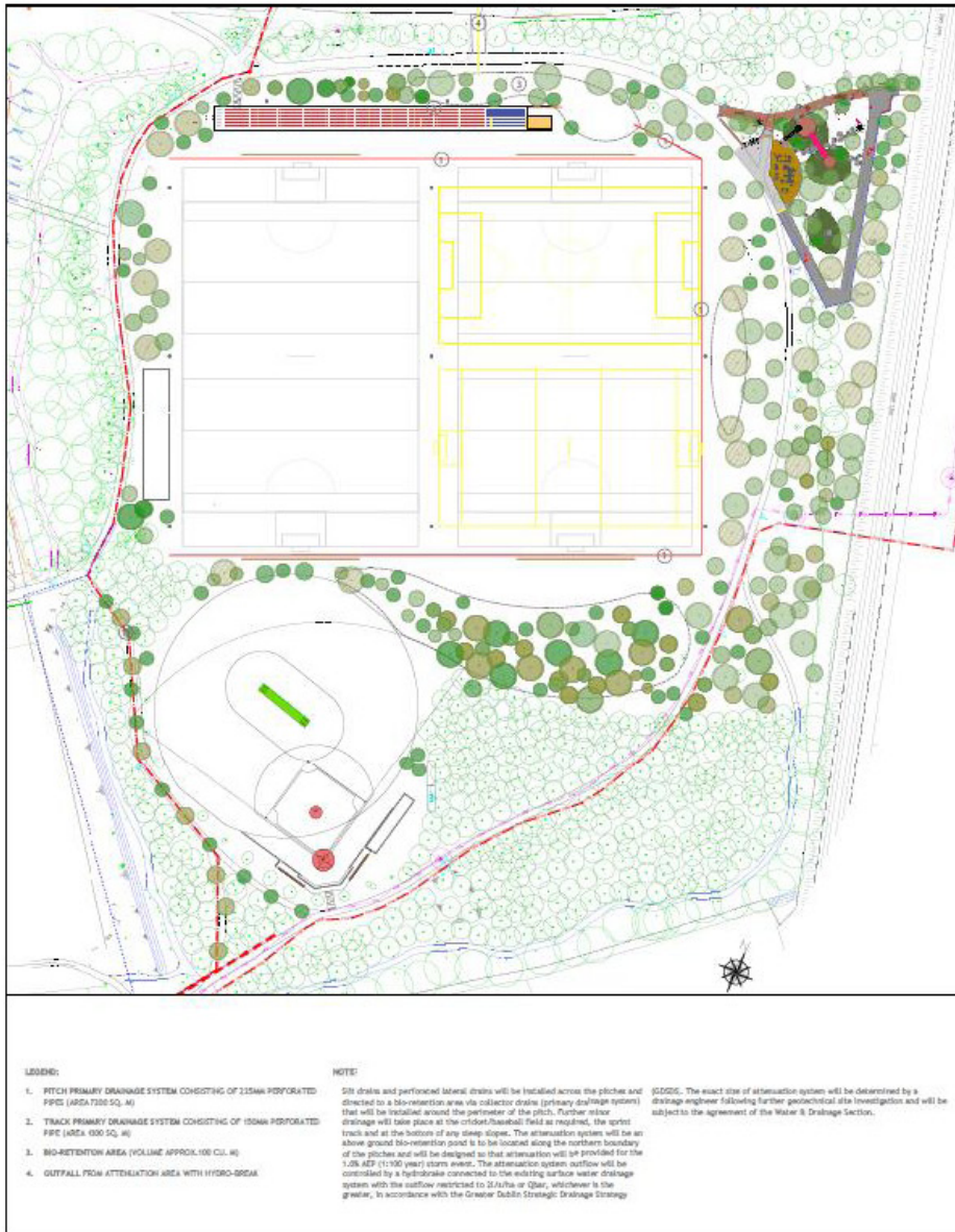
Figure 3 Site Drainage – Drawing no DRP 2422-12
