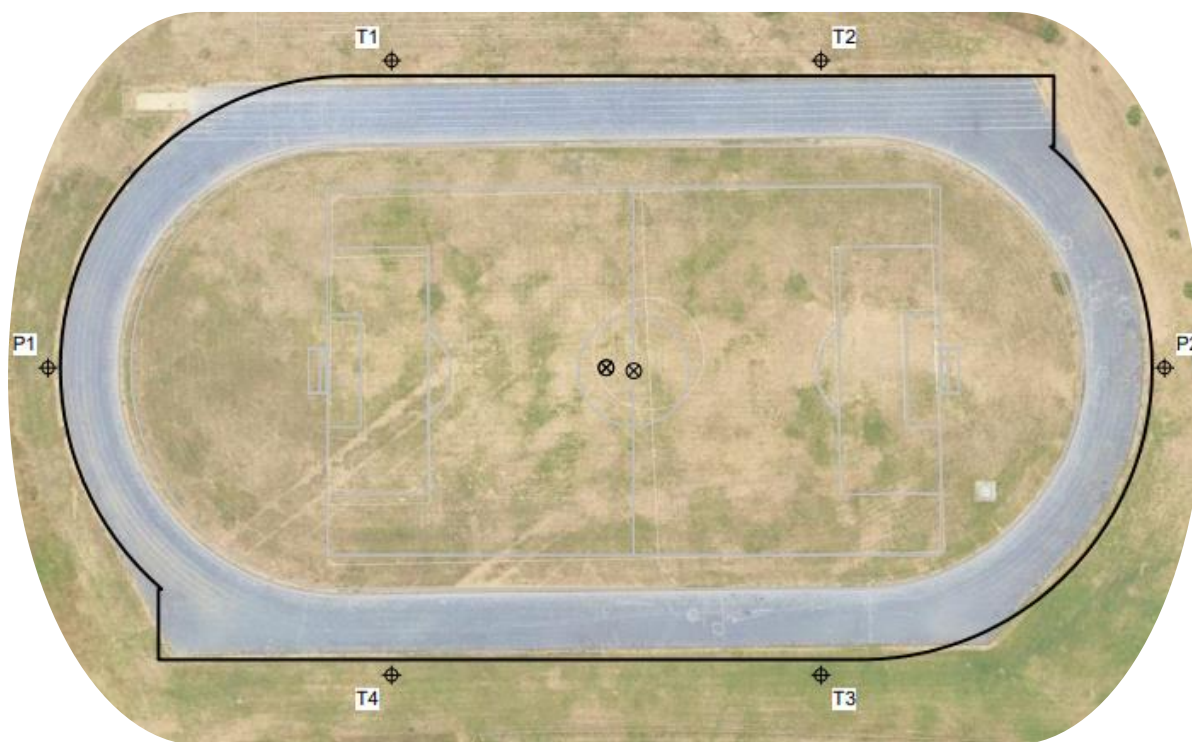
Figure 11: Position of columns around the Kilbogget athletics track (Source: Musco Lighting)
