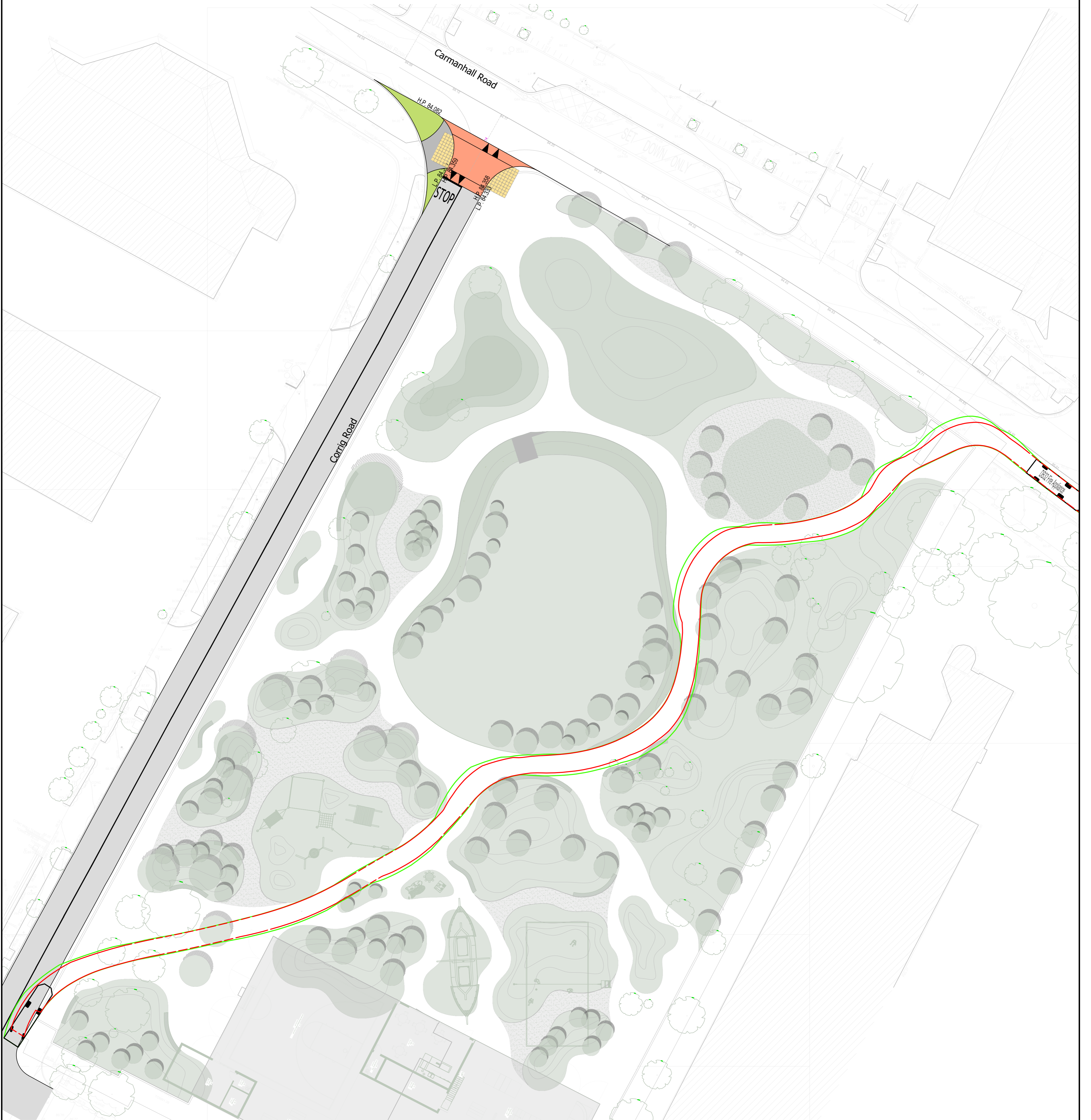
PROPOSED FIRE TENDER VEHICLE TRACKING THROUGH PARK SCALE 1:250
