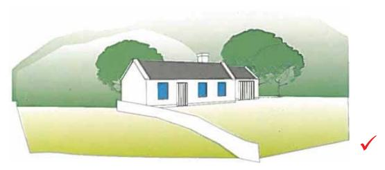
A garage will often look better set back to read as separate structure whilst still having a physical connection. This can help to reduce bulk and emphasis that the house is the more important structure on site.
