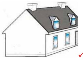
Consideration should be given to using roof space for bedrooms where 2-storey dwellings are sought. This can reduce bulk and scale and provide dormers that successfully integrate into the roof from the outset.
