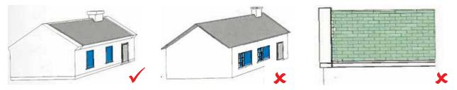
Using a more traditional form, the gable holds the roof and gives it a functional and secure appearance
