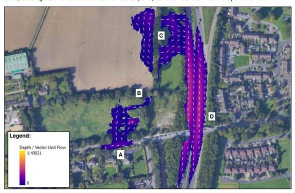
Figure 6-14: 0.1%AEP MRFS - Overland Flow Path Directions
