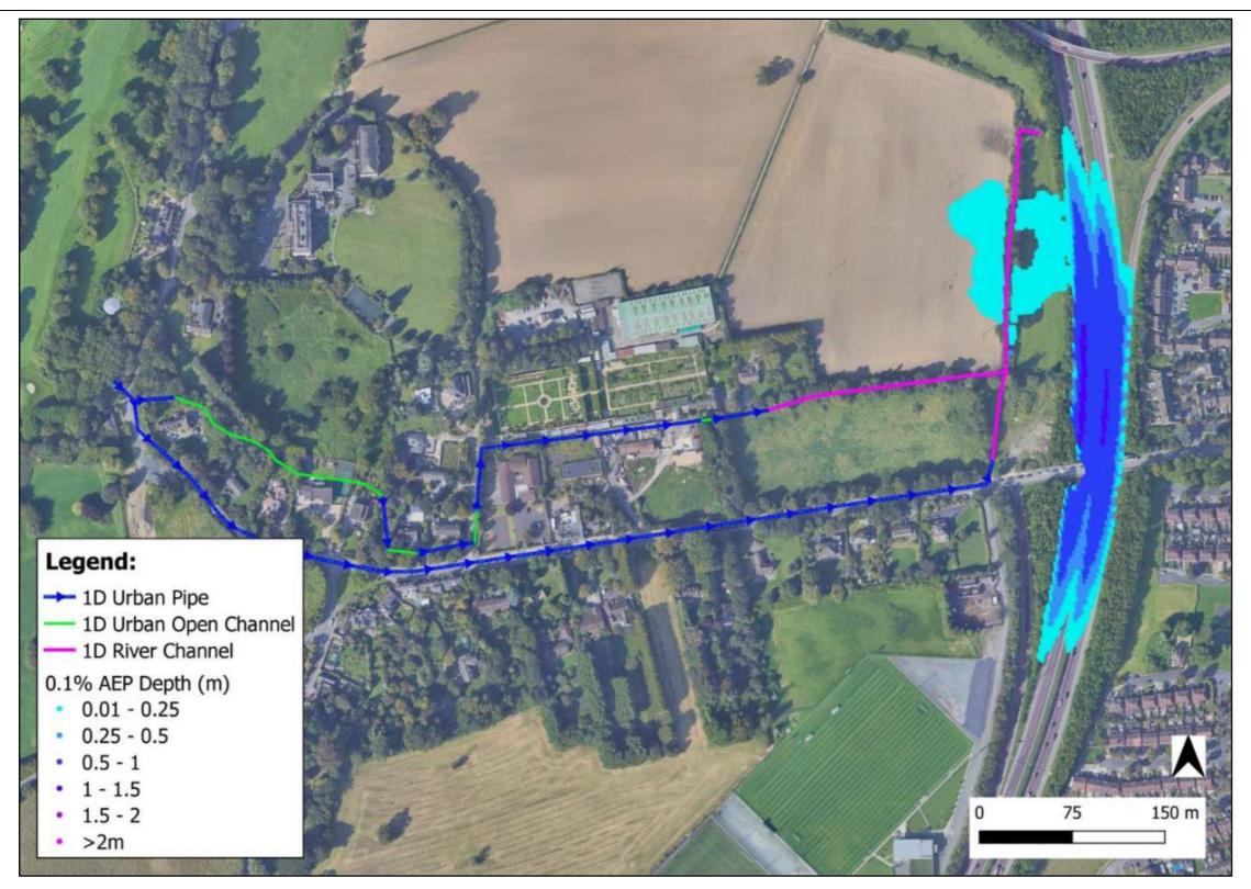
Figure 6-8: Current Scenario 0.1%AEP Flood Depth
