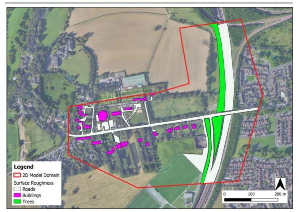
Figure 6-5: Tuflow 2D Domain Surface Roughness
