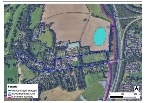
Figure 4-9: Pluvial Flood Risk Area Identified by Landowner
