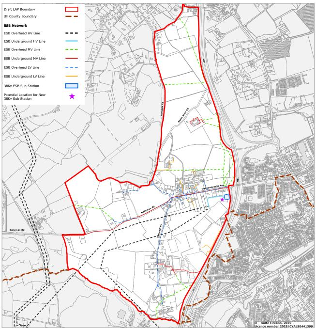
Figure 10.8: Electricity Network in the LAP area (Indicative Only, refer to ESB for ESB Network)
