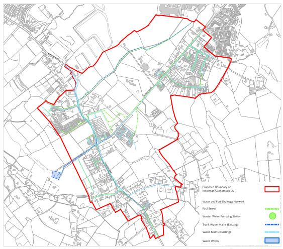
Figure 13.1: Water Supply and Foul Drainage Network within the LAP Area
