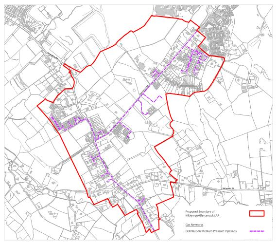
Figure 13.3: Gas Network within the LAP Area
