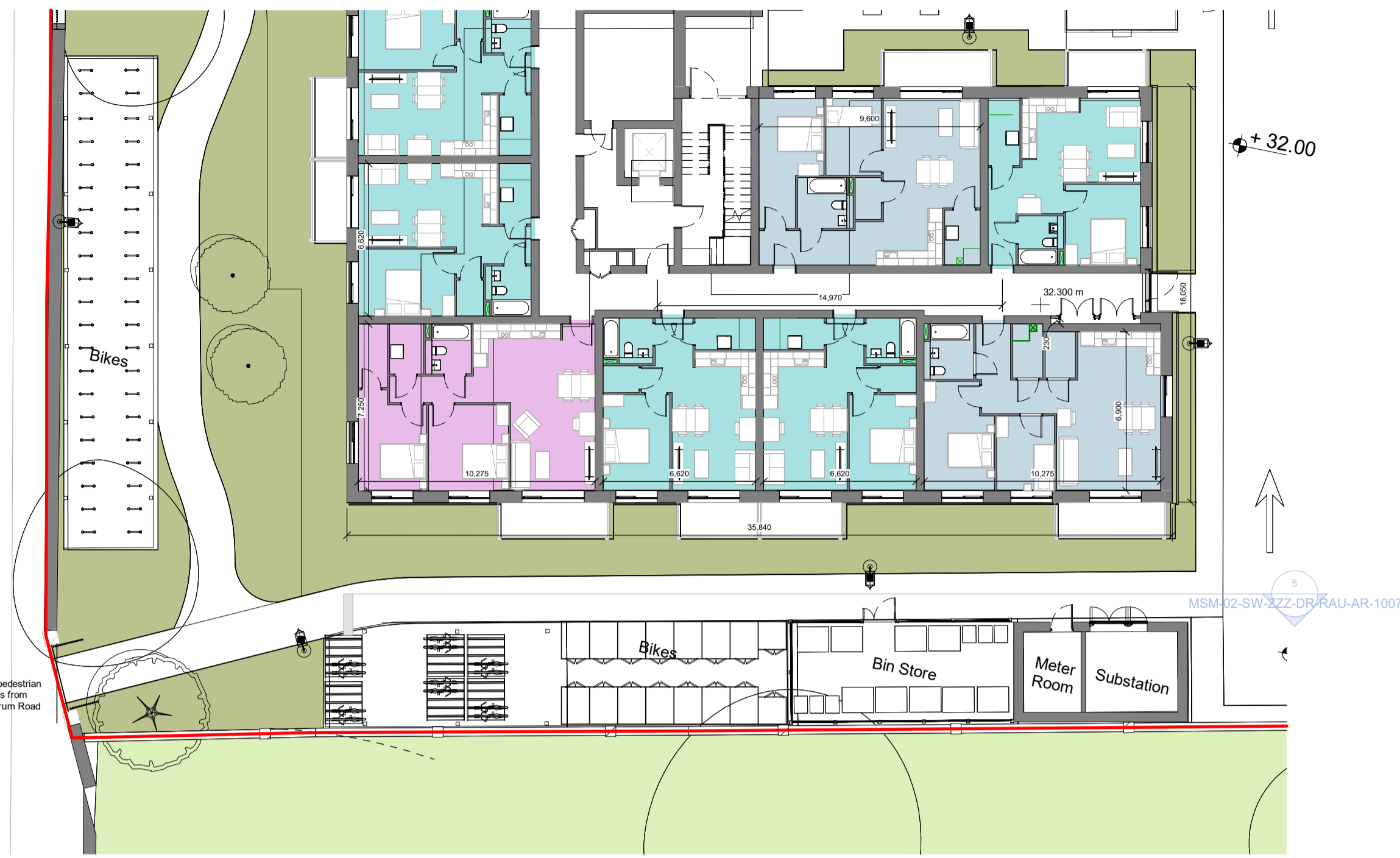
L00 Block A - Bin Waste Store, ESB Substation, External Storage & Covered Bike Shelter 1 : 200
