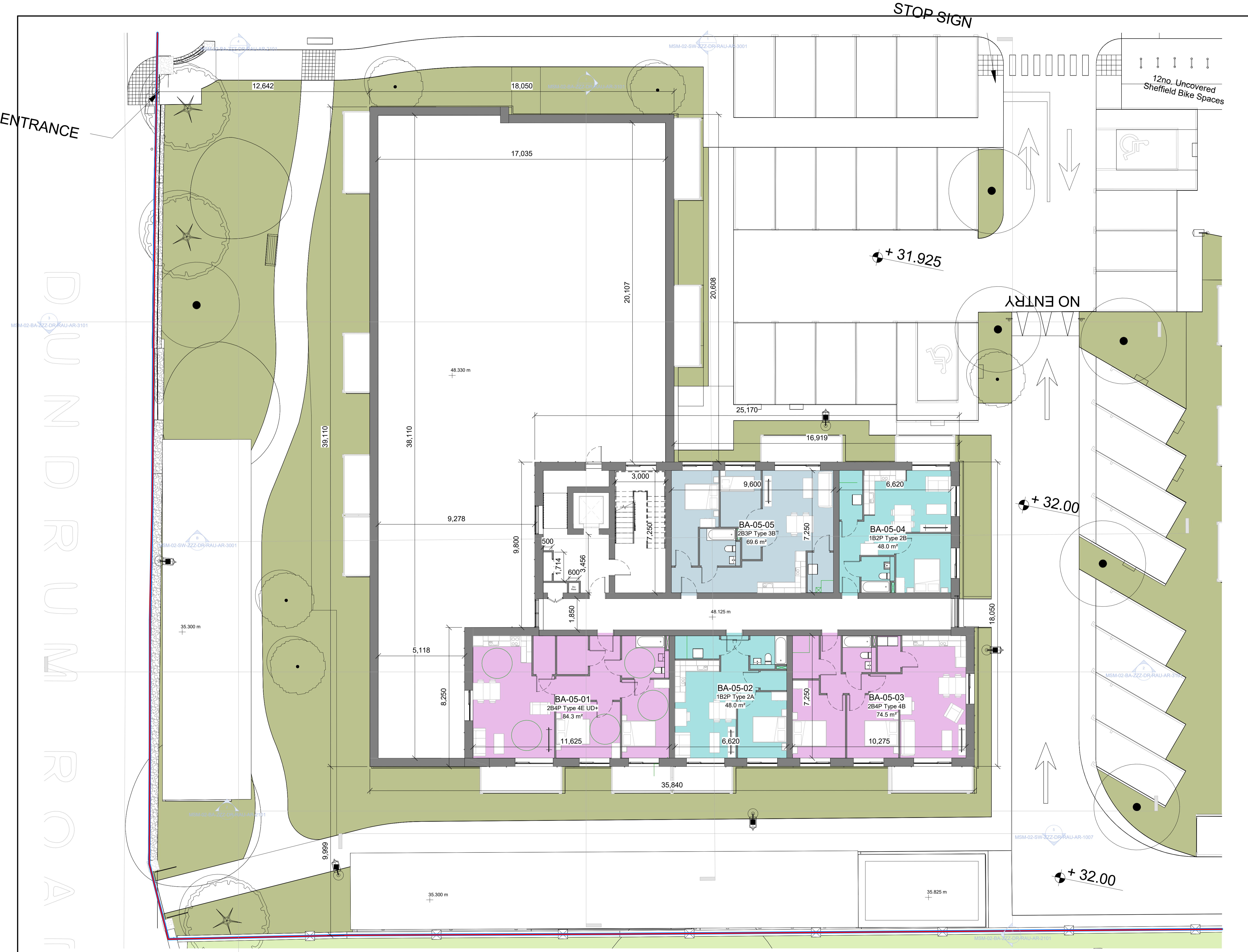
L05_Block A Fifth Floor Plan 1: 100
