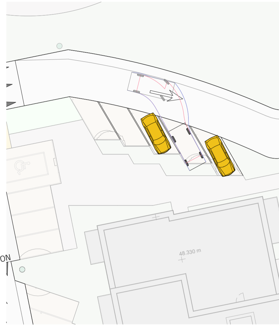
CAR AUTOTRACKING 4 OUT 1: 250
