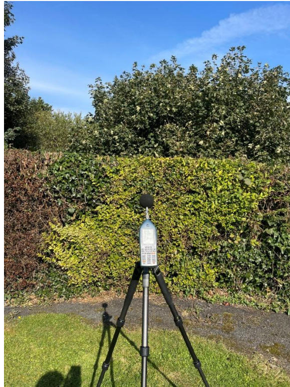
Figure 5: Attended Noise monitor Setup
