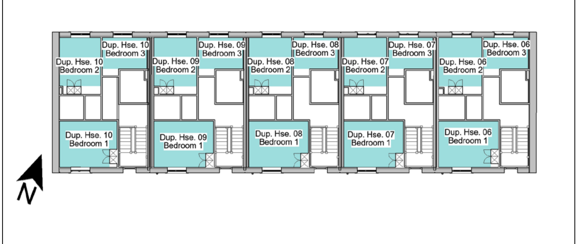
Figure A.4: Duplex Terrace 1-5 - Level 02
