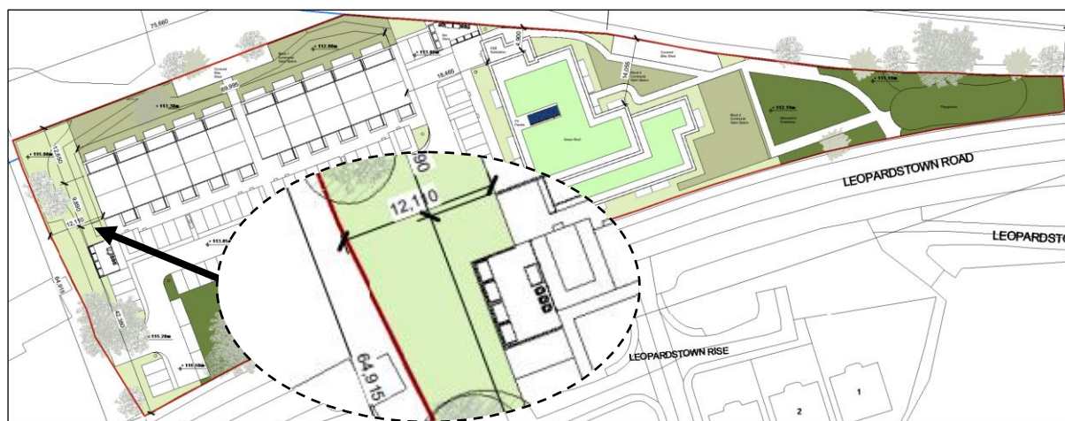
Figure 50.0 Proposed site layout plan demonstration separation distances between the subject
