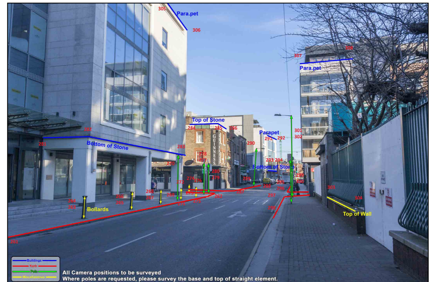
Fig.8: Fixed reference points surveyed and numbered by surveyor.
