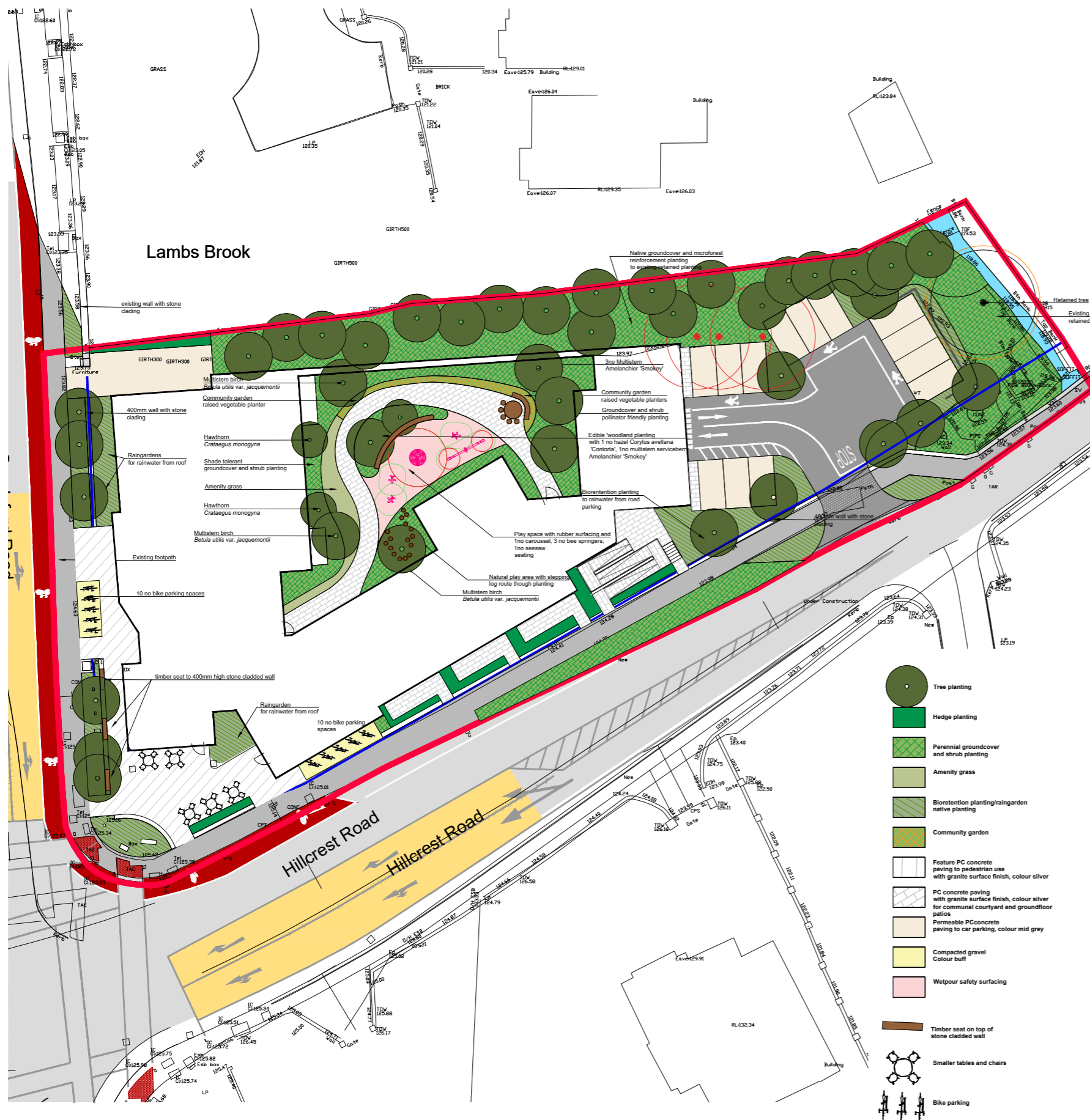
Image 37: Landscaping Plan prepared by Mitchell + Associates illustrating the layout both at ground level around the external perimeter of the block and the first floor roof garden that serves as the communal amenity space for the development
