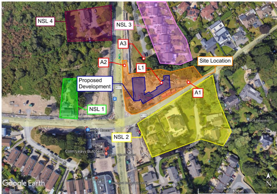
Figure 14: Site location and noise sensitive locations 1-4.
