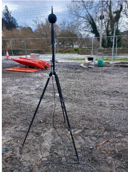
Figure 5: Attended Noise Measurement Setup
